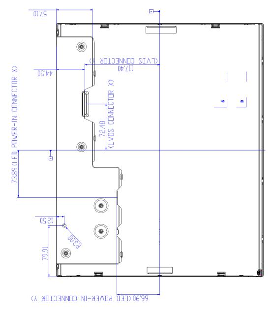
(NOTE: Two LED backlight power cables are not shown)
