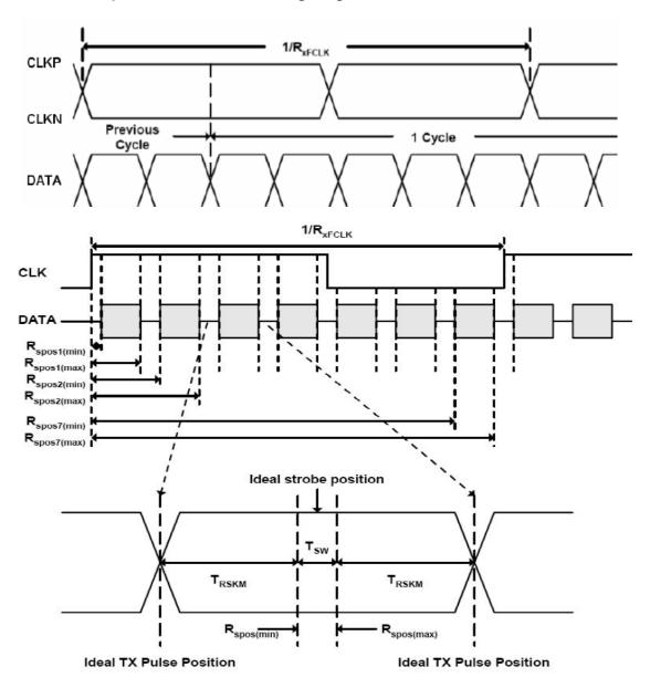
T<sub>RSKM</sub>: Receiver strobe margin R<sub>SPOS</sub>: Receiver strobe position T<sub>sw</sub>: Strobe width (Internal data sampling window)
